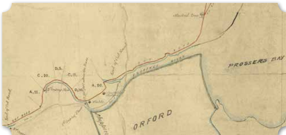
Figure 3. Part of a plan showing the route of the convict road at Orford. Undated, but possibly 1850s or early 1860s. It is in fact partly incorrect; the route shown north of the river at C10 to D10 was not built, but rather the road crossed to the south side between the 'second crossing place' and the 'first crossing place' cutting off a cliffy bend in the river. Note also in light pencil the new route south of the Prosser on the left, indicating the date of the map. The Probation Station lay between 'D10' and 'A26' and is not shown, indicating that it had been closed. Portion of Tasmanian Archives plan AF398/1/1.
